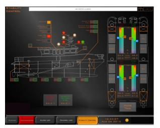
Ship trim and draught conditions can be easily evaluated and optimised using Servowatch's new ServoTrim system
